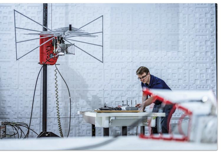
Before any digital electronic or radio-enabled product can be placed on the market, it must be assessed to ensure it meets the relevant regulatory compliance requirements. These requirements vary per region but may include topics such as product safety, electromagnetic compatibility (EMC), radio performance, radio system efficiency, and interoperation with other services.
