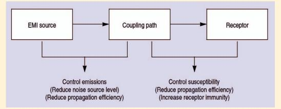
Electromagnetic interference is a major problem in modern electronic circuits. To overcome the interference, the designer has to either remove the source of the interference, or protect the circuit being affected. The ultimate goal is to have the circuit board operating as intended – to achieve electromagnetic compatibility.
